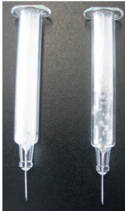
Fig. 8: Glass dust test: left – syringe siliconizea with an diving nozzle, right – syringe siliconizea with a fixed nozzle.
