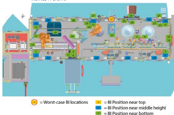
Figure 5: Isolator BI Locations versus D-value using direct injection © METALL+PLASTIC
