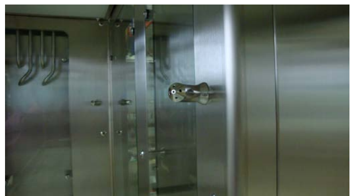
Figure 3: Position of a direct injection nozzle in production isolator © METALL+PLASTIC
