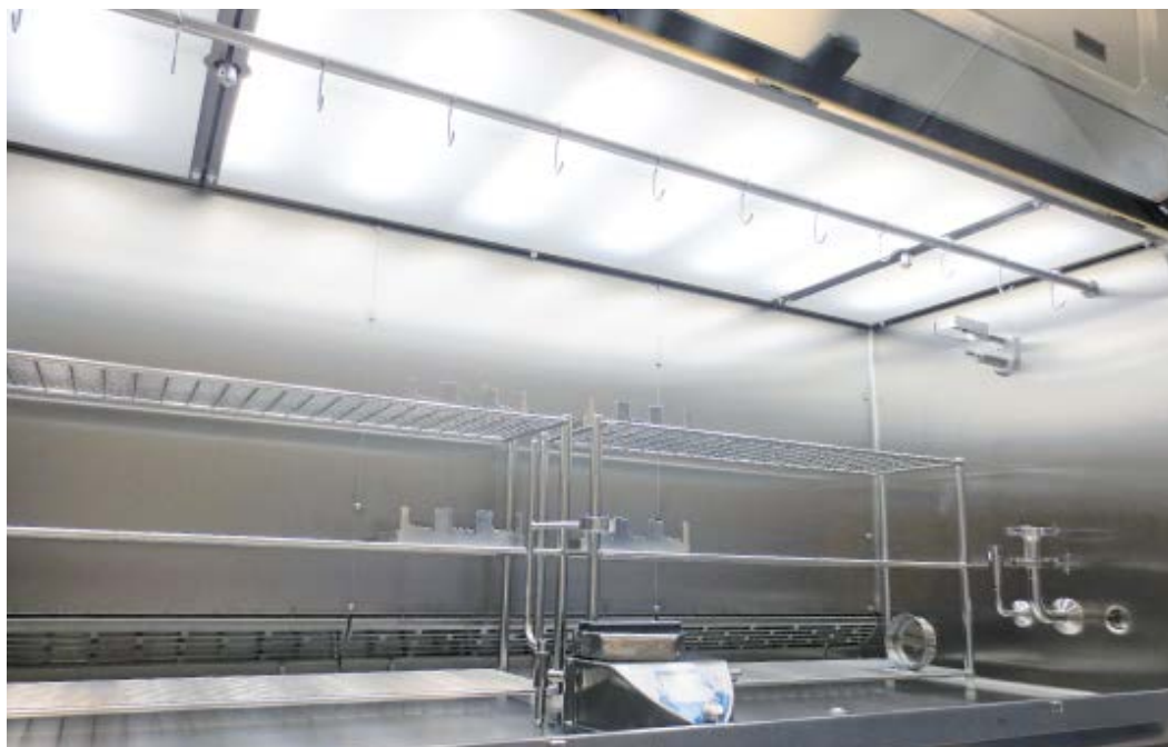
Figure 1: direct injection nozzles installed as a bypass of the CG membranes © METALL+PLASTIC
