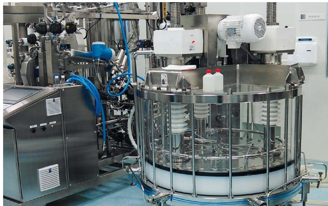
Figure 1: VERDOT Ips<sup>2</sup> InPlace™ Chromatography Column
