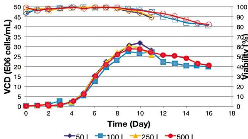
*The following data represents a fed-batch culture with CHO-S grown in Dynamis and Efficient Feed C+ Media in the 50L, 100L, 250L, and 500L SUBs. Cultures were initially seeded at 20% WV and scaled to full working volume on day 2 or 3 of culture. Growth rates and productivity levels were maintained across 4 different systems representing a full magnitude of scale-up.*
