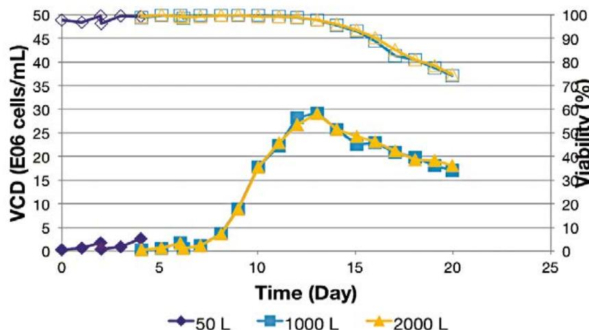
*The following data represents the 50L 5:1 SUB starting at 10L, expanding to 50L, and then seeding into parallel 1000L 5:1 and 2000L 5:1 SUBs in this fed-batch CHO-S qualification run.*
