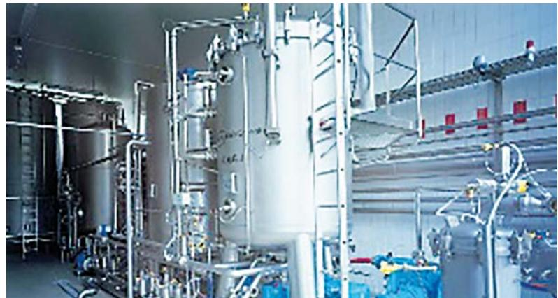
The Cadence BioSMB Process system is capable of processing HCCF from bioreactors as large as 2,000 L under cGMP conditions at flow rates of up to 350L/h. The Cadence BioSMB Process system also has a single-use flow path and leverages the design established for the PD unit.
