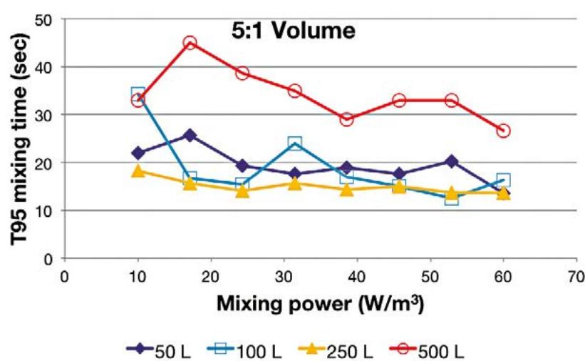
*The following data represents t95 mixing times of the 50L 5:1 SUB at 10L, 100L 5:1 SUB at 20L, 250L SUB at 50L, and the 500L 5:1 SUB at 100L.*
