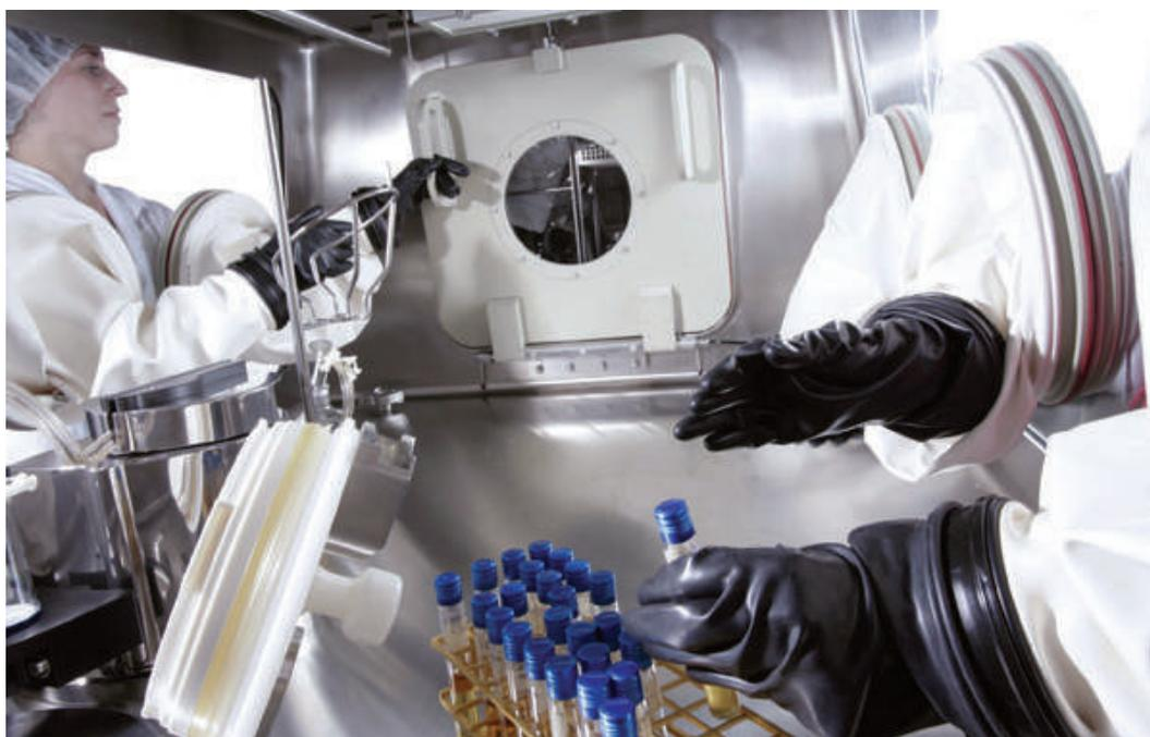
Besides, the gloves which are used to supply the crucial interface between the interior isolator environment and the worker. The integrity of the gloves is critical, so a glove breach is a breach in containment that puts products and/or workers at risk of contamination. Therefore, prevention and detection of breaches in gloves and sleeves during manufacturing operations is a key aspect of the maintenance of the barrier against contamination of the Grade A environment.
