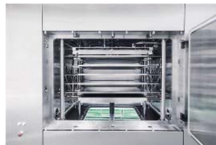
↑ Figure 2 : Freeze-drying of plasma derivatives has become the preferred method for preserving sensitive coagulation factors.
