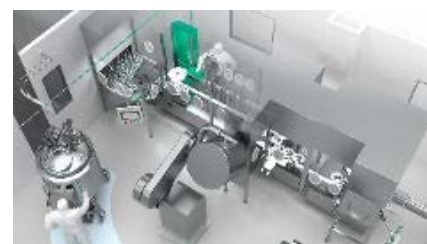
↑ Figure 1 : Sensitive plasma derivatives are typically filled in isolators or RABS systems to ensure their safety.
